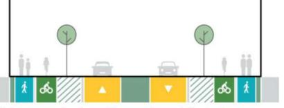
The berm space and median would be removed on any bridge structure
